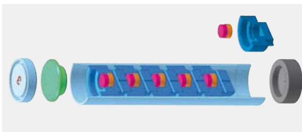
Diagram of the experimental irradiation device for transmutation in americium-bearing blankets.
