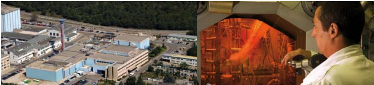
Minor actinide separation test in the hot laboratory Atalante.
